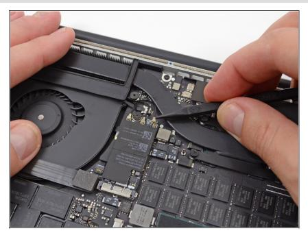
Use the tip of a spudger to pry the three AirPort antenna cables straight up off of their sockets on the AirPort board.
